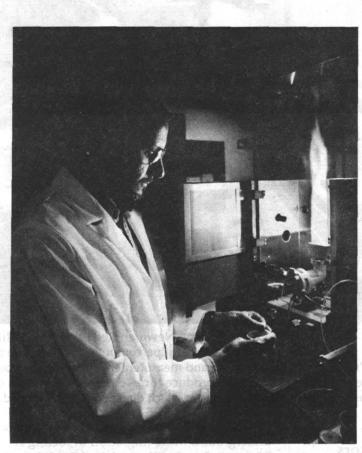
CHEMICAL ANALYSIS - Mike Courtney (14466) uses an atomic absorption spectrometer to conduct chemical analyses of neutron tube target and sources. Here the flame from the spectrometer is visible. A broad range of chemical analyses are used to support neutron tube and generator processing.
